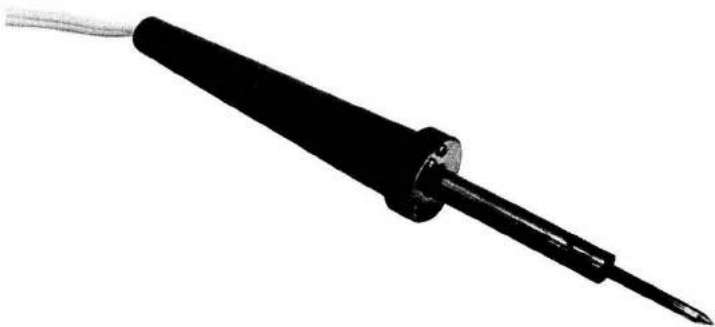
Fig. 3-22. A 30-watt soldering pencil suitable for most electronic soldering.
