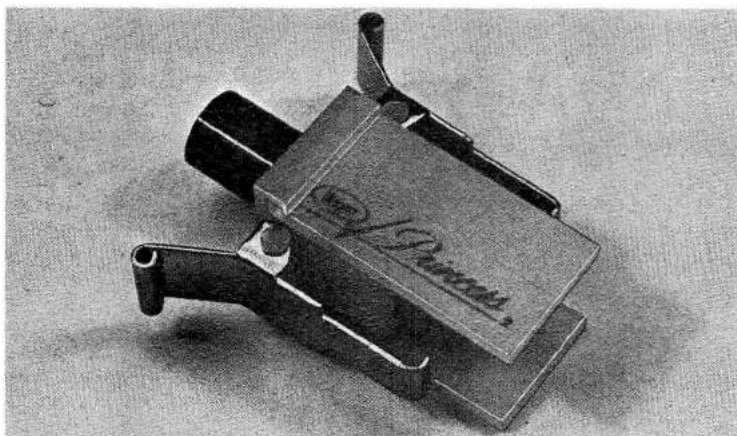
Fig. 5-7. DIP desoldering clip. The metal clips go under the ends of the DIP package. When the solder joints are melted, the DIP is pulled away from the PC board.
