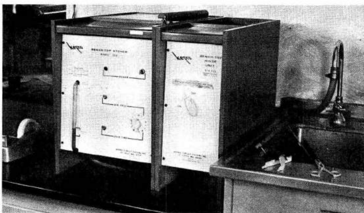
Fig. 3-18. The etching unit at the left will handle double-sided boards up to approximately 8" × 12". The unit at the right is a water-spray rinser which removes etching solution from the finished board.
