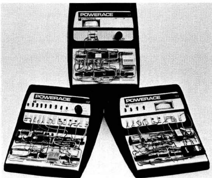
Fig. 2-2. Modern breadboards or circuit designers with built-in power supplies and other functions. Notice that the model at lower left has many functions, such as bounceless switches and various clock frequencies useful in digital applications. (Courtesy AP Products Inc.)
