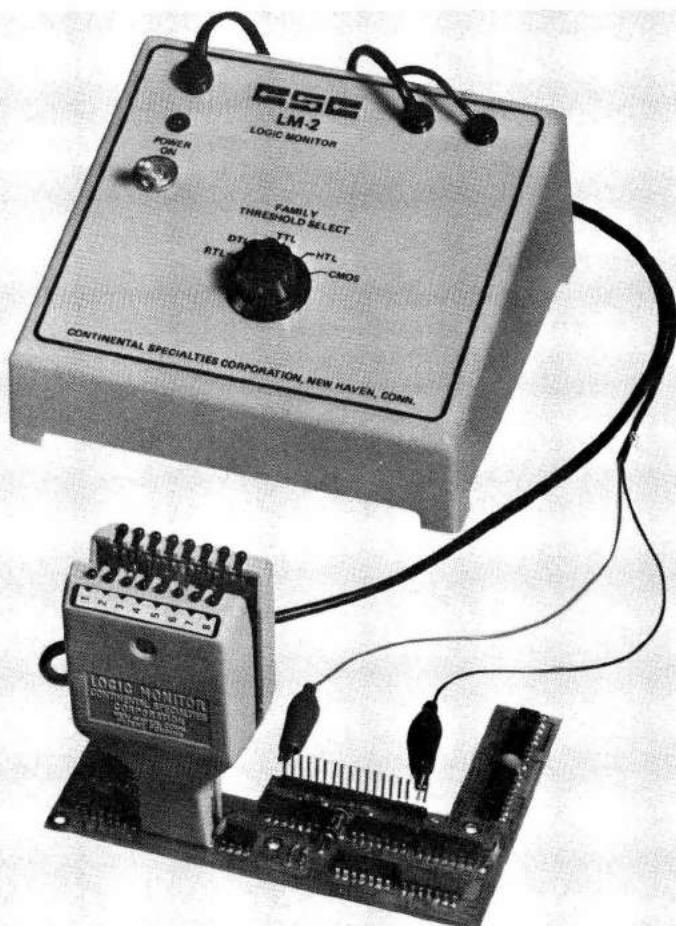
Fig. 5-11. Logic monitor with its own power supply. The power supply can be set for any one of five logic families. (Courtesy of Continental Specialties Corp.)
